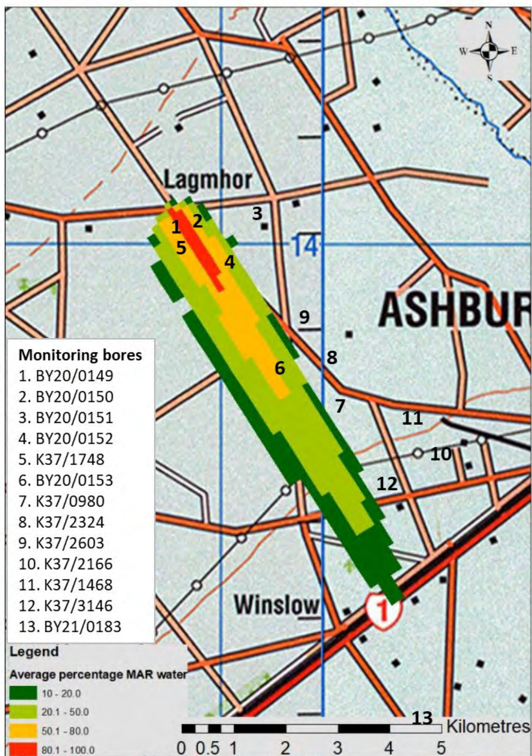
Figure 4-8: Modelled groundwater quality change after 5 years in response to the MAR trial (from Durney, 2019, Figure 5-23 MAR plume Layer 3)
