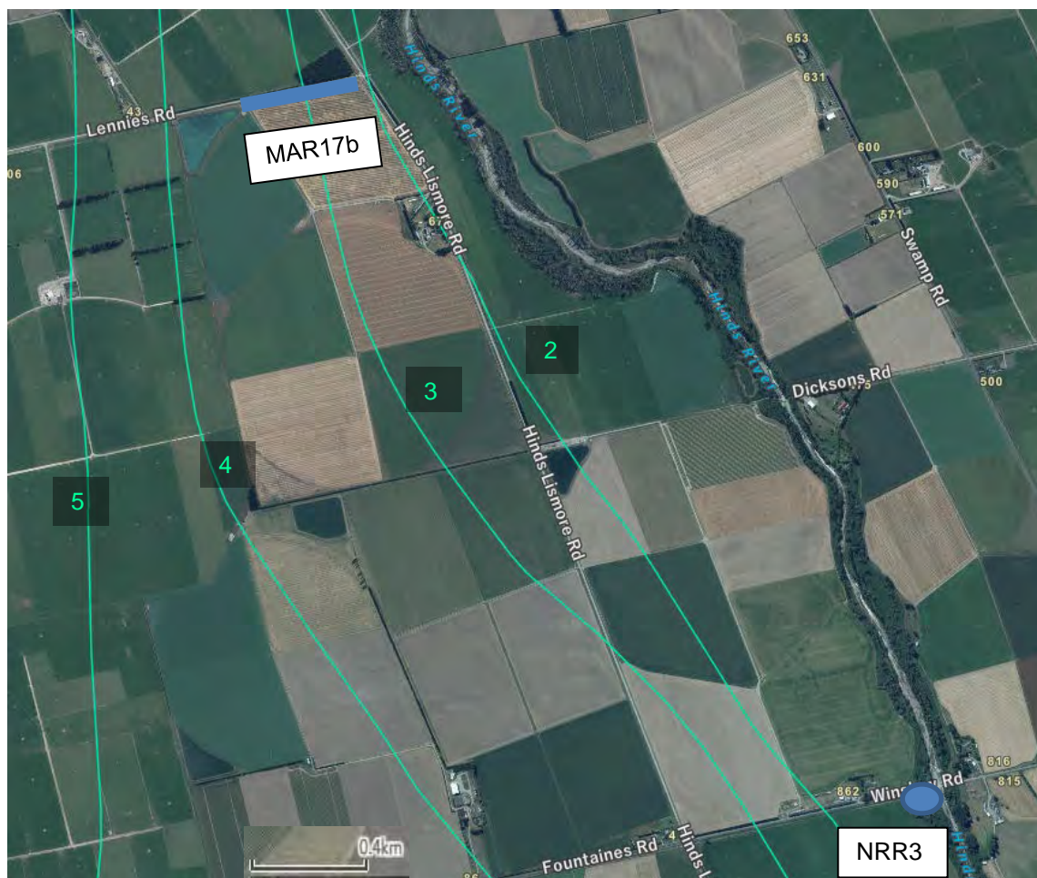
Figure 2-21: Location of MAR17b and proposed NRR3, plus minimum depth to groundwater contours (in m) (Source: Canterbury Maps)
