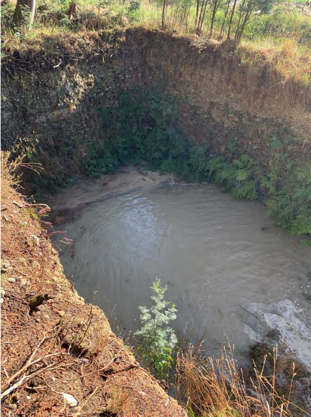
Figure 5-12: MAR Site 18, McDougalls Road (infiltration testing prior to backfilling)
